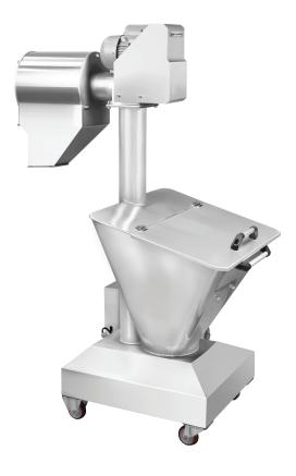
MSM50 Flour Sifter is a very useful machine for bakeries, hotels, restaurants and pastry shops. The main function of the flour sifter is to remove all lumps in the flour to obtain a soft dough and also to remove foreign materials that may be contaminated by flour bags. Flour sifters also improve product quality by allowing better oxygenation of the flour.
