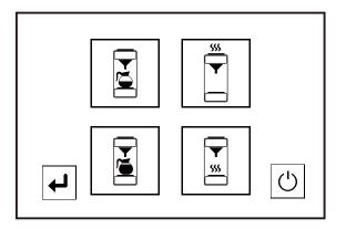
Press the following button to switch ON the upper warming plate. Press this button again to switch OFF the upper warming plate.
