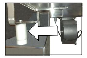
Place the nozzle of the tempering machine upon the half-moon chocolate dispenser (it is possible to regulate it using the buttonholes). Note that the chocolate flow tends to fall in the nozzle direction and not perfectly in the center
