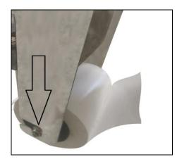
The paper must pass above the stainless steel bar connecting the two white feet, and on the right of the stainless steel round tube. Then insert the paper between the detailer and the last section of the enrober.
