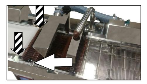
It is possible only a small regulation of the detailer. The two knobs for the setting of the detailer must be both in the same position, with the same angle, so the rotation axis is perfectly straight to the motor. Place the hopper on the specific supports.
