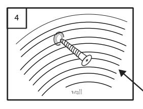
Securely attach 2 screws into the wall plugs.
