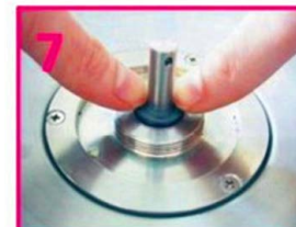
Put the airproof ring along the motor revolving axle. And clean the remaining lubrication oil.
