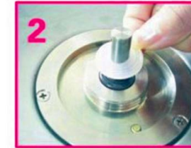
Take out the silica gel ring from motor revolving axle
