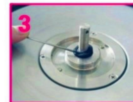
Please use thin metal stick to pick up the airproof ring out (don't touch the Motor Revolving Axle)
