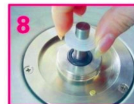
Put the new silica gel ring in to the machine
