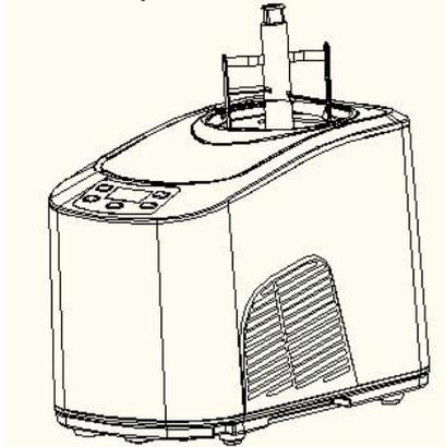
4/ Put back the transparent cover and turn it clockwise to install tightly. Then plug in the unit.
