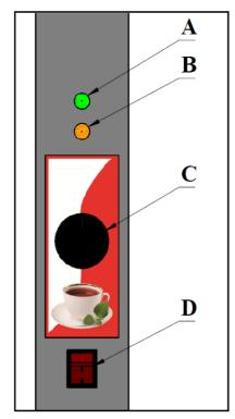
A: Indicator lampB: Indicator lampC: ThermostatD: 0-1 Switch
