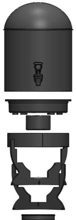
Throw in two legs ( No:3 + No:4). Place inside to receptacle of induction heater (No:5 ) and Induction heater ( No:6).
