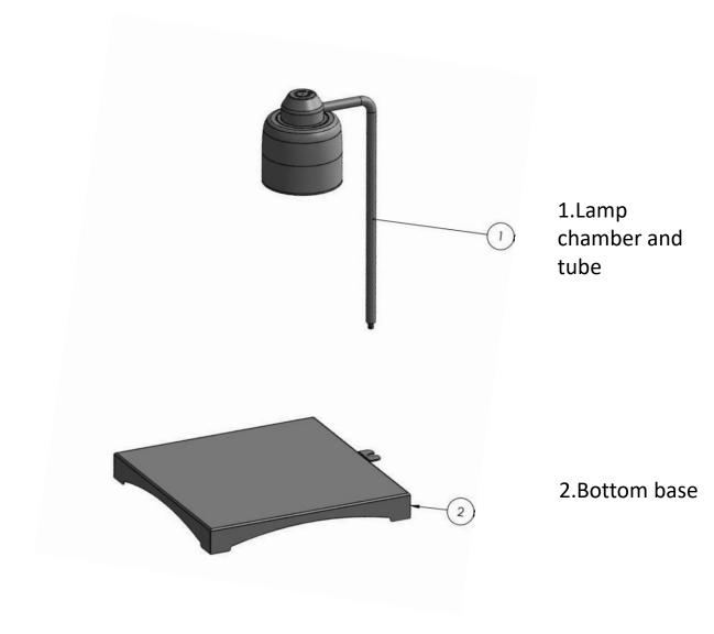
Connect the pipe (No:1) to the subbase(No:2) by tightening the strip with the wrench.
