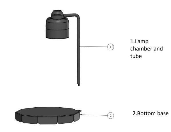
Connect the pipe (No:1) to the subbase(No:2) by tightening the strip with the wrench.
