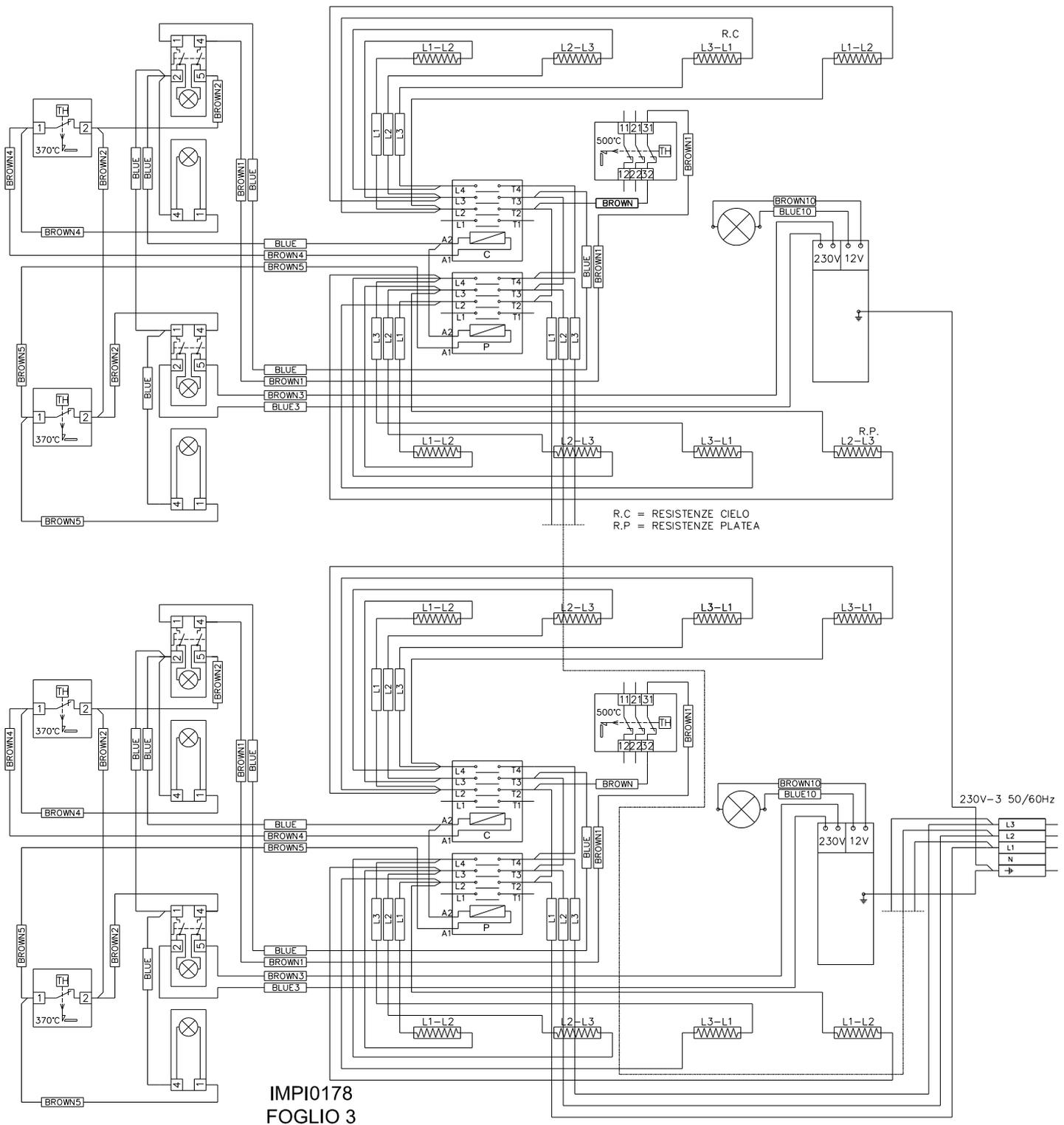
Fig. 8.5. Electrical diagram Citizen EP70 double chamber, at 230 Vac. 3 version.
