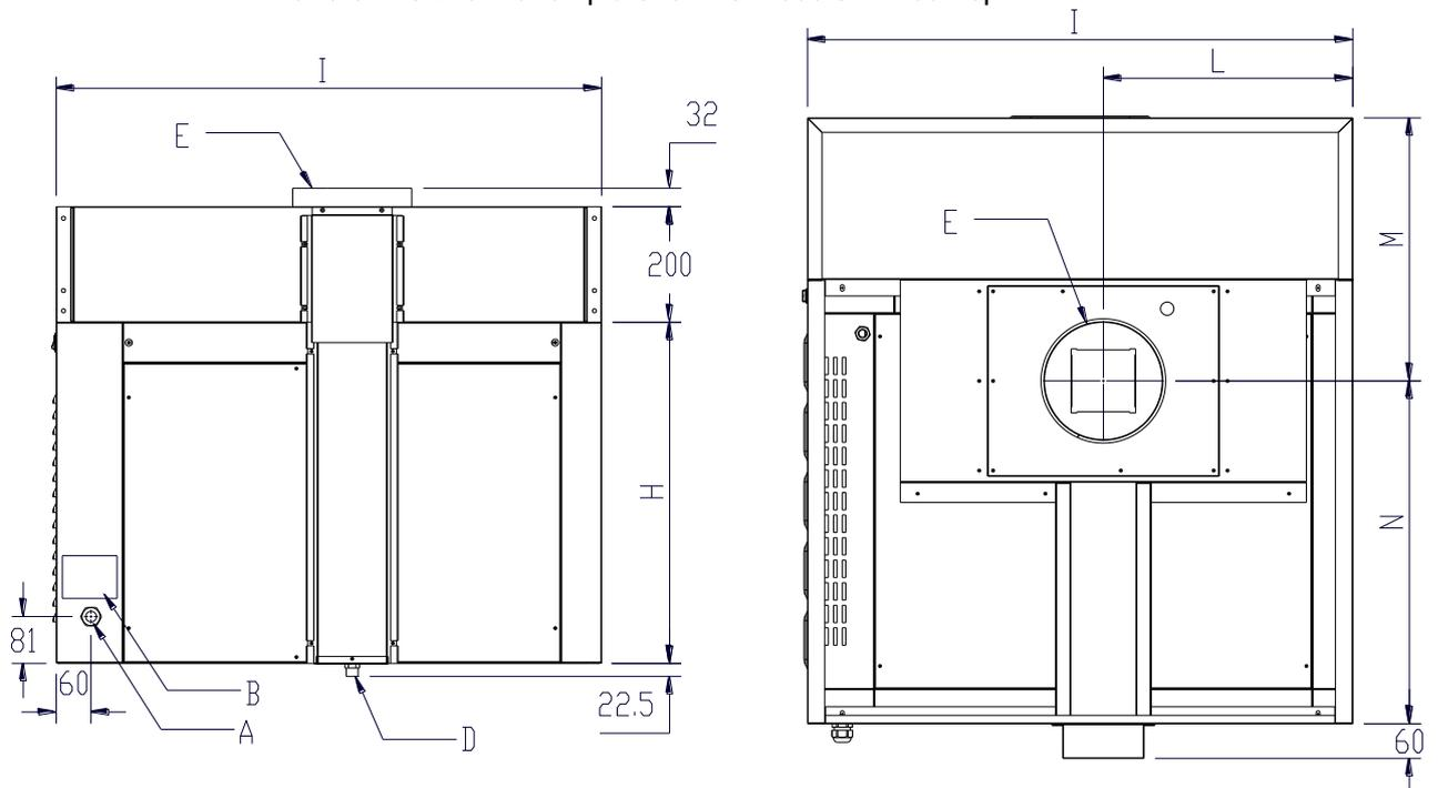
Fig.4.5 Point of entry for the electrical cable, the vapour exhaust outlet, the condensation exhaust outlet and of the information plate for the module with a top.
