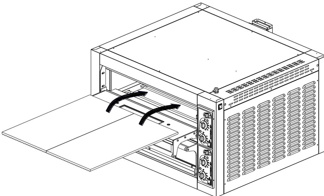
**N.B. Insert the refractory surfaces with the corrugated surfaces facing downwards.**
