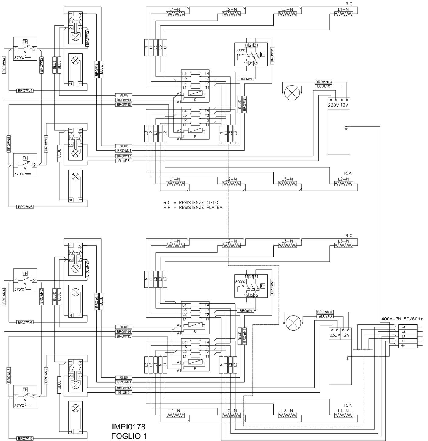
Fig. 8.4. Electrical diagram Citizen EP70 double chamber, at 400 Vac. 3-N version.
