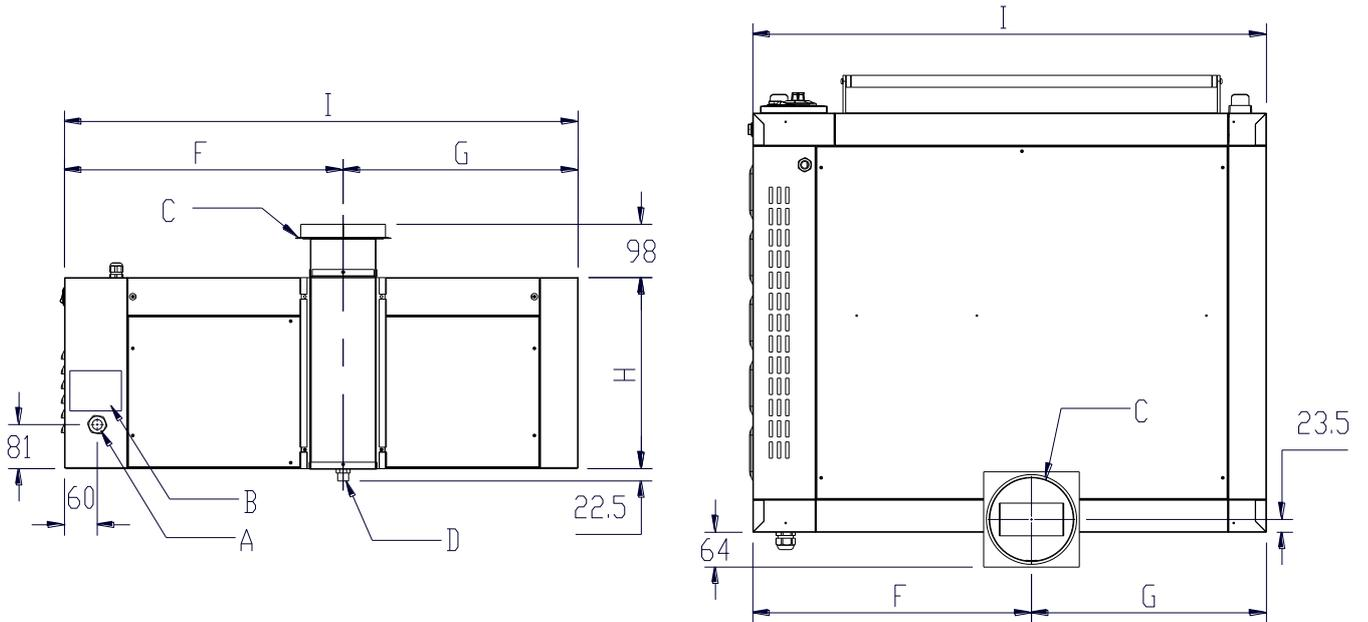
Fig.4.4 Point of entry for the electrical cable, the vapour exhaust outlet, the condensation exhaust outlet and of the information plate for the module without top.
