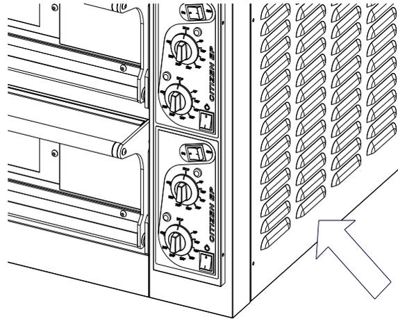
Figure 4.1. Cooling openings
