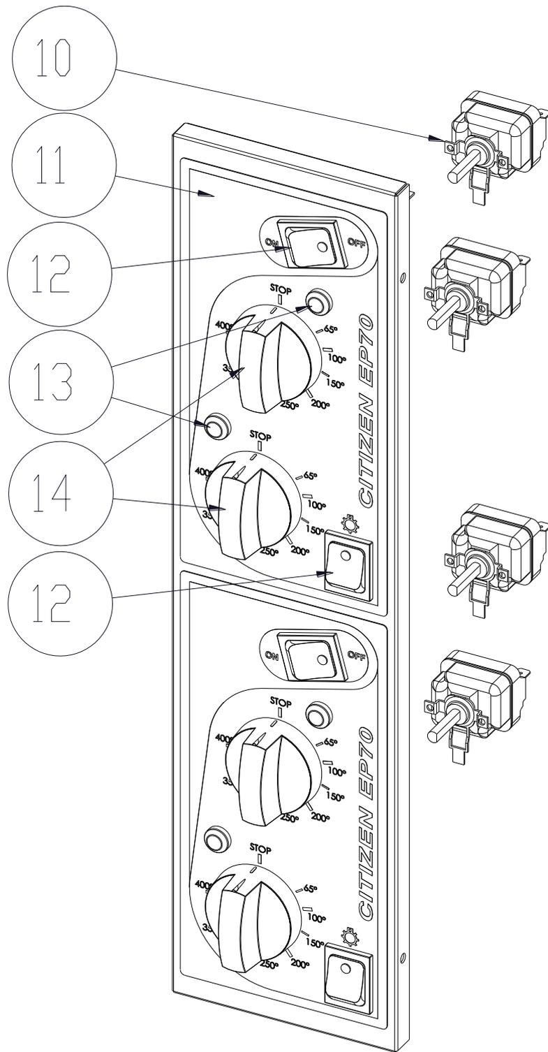
Figure 8.9 Exploded view of electrical parts
