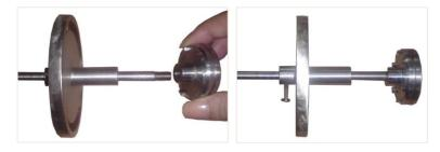
3. Screw the plunger with the matched mold.
