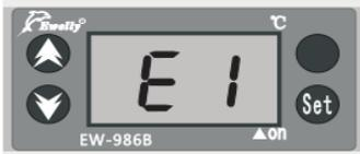
ON Error: when the sensor is short circuit. Code “E1” will be displayed.
