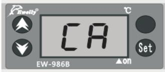
Press **set** key, then press **▼** or **▲** simultaneously. Choose temperature correction:  $-15^{\circ}\text{C}\sim 15^{\circ}\text{C}$
