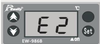
When current temperature is higher than the upper limit, the screen will display “E2” and the load will be off.
