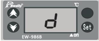
Hold **set**, then press **▼** or **▲** simultaneously. Choose return difference:  $1^{\circ}\text{C}\sim 15^{\circ}\text{C}$
