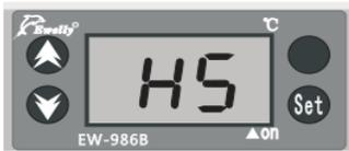
Press **(set)** key, then press **(▼)** or **(▲)** simultaneously. Choose high-est temperature limits: control temperature+1°C ~400°C
