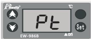
Press **(set)** key, then simultaneously press **(▼)** or **(▲)** to set delayed star time from 0 to 3 minutes.
