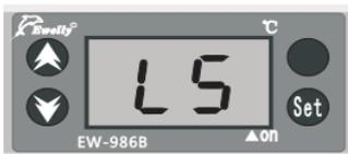
Press **(set)** key, then press **(▼)** or **(▲)** simultaneously. Choose lowest temperature limits: 0°C ~control temperature-1°C
