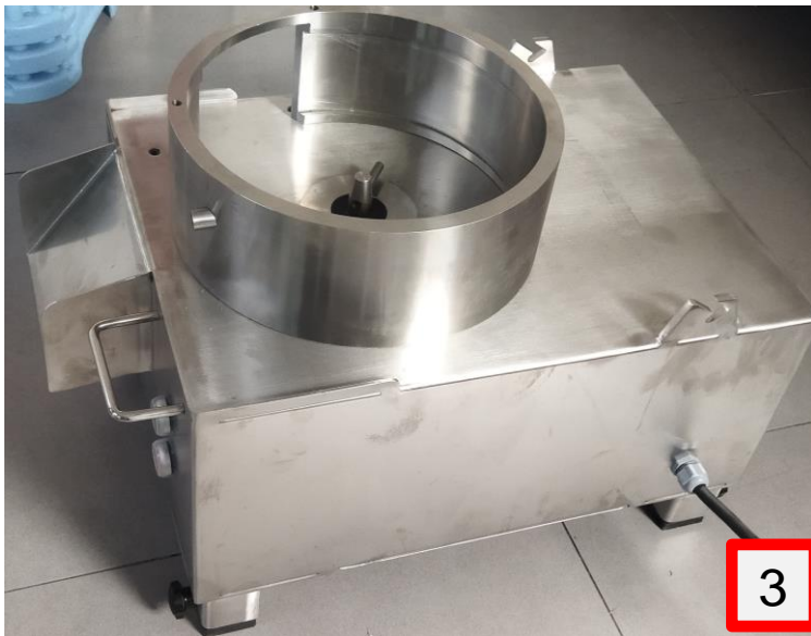
[ 3 ] – Remove the Pusher Disc Drum
