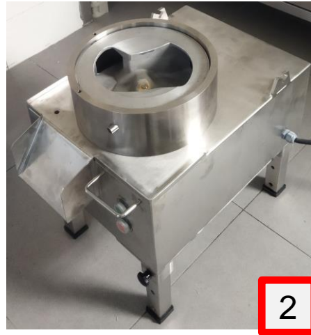
[ 2 ] – Remove the Blade Block Group
