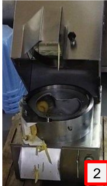
[ 2 ] – Open the feeding hopper
