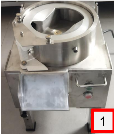
[ 1 ] – Remove the feeding hopper
