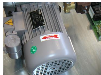
Image 5.2. Adhesive labels indicating the rotation direction.
