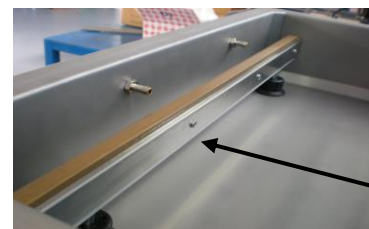
Image 8.1. Sealing bar within the chamber
