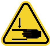
Warning: Danger of Hand Caught
