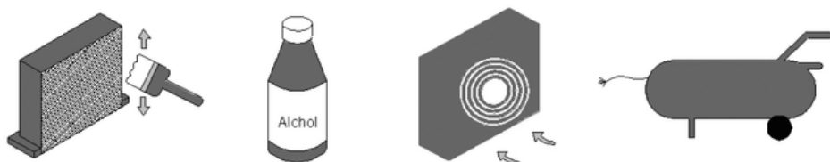
Figure 6 Cleaning of the Condenser
