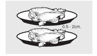
Position trays inside the tray compartment as far as they will go, as close as possible to the evaporator.
