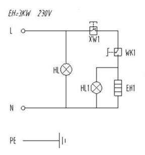
WK1- temperature controller XW1-temperature limiter
