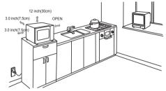
The rear surface of appliance shall be placed against a wall.
