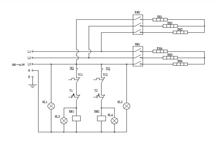
KM: AC Contactor; EH Heater; SQ Switch; T: Thermostat; TCL: Temperature Control Limit; HL1-2: Power Indication Light; HL3-4: Working Indication Light
