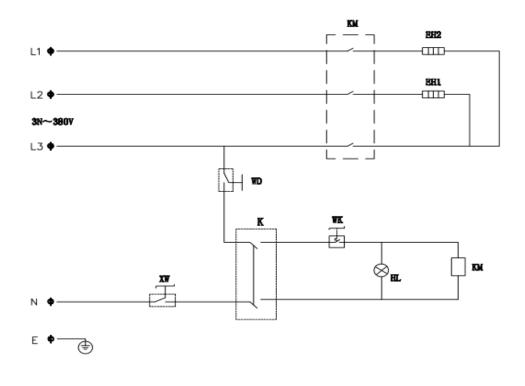
WD----Touch switch EH1、EH2---Element K---Switch HL---Heating light KM---Ac contactor XW---temperature limiter WK---Thermostat
