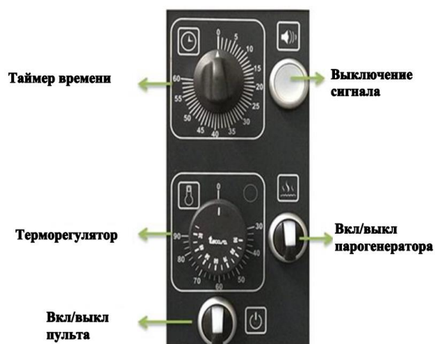
Figure 4.4. Proving cabinet climate control panel
