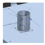
Outward bend the 4 fins placed on the chimney for fumes discharge of the equipment, in order to obtain a support for the pipe of the channeling.
