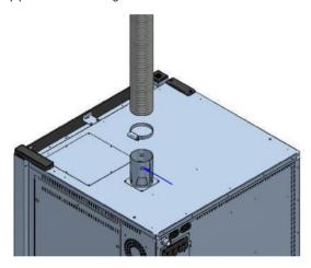
Connect the channeling pipe to the exhaust pipe of the unit and secure it through an adequate metal clamp.
