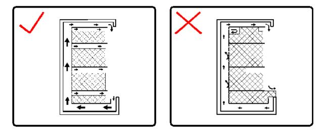
Failure to enable cold air to circulate as designed can lead to product temperature not being maintained and affects the functionality of the cabinets refrigeration system. When loading frozen products wear insulated gloves.
