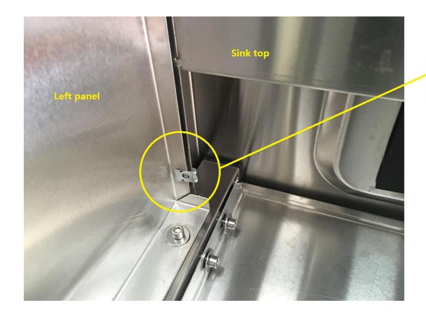
Put the connecter to hold the left panel and sink top.
