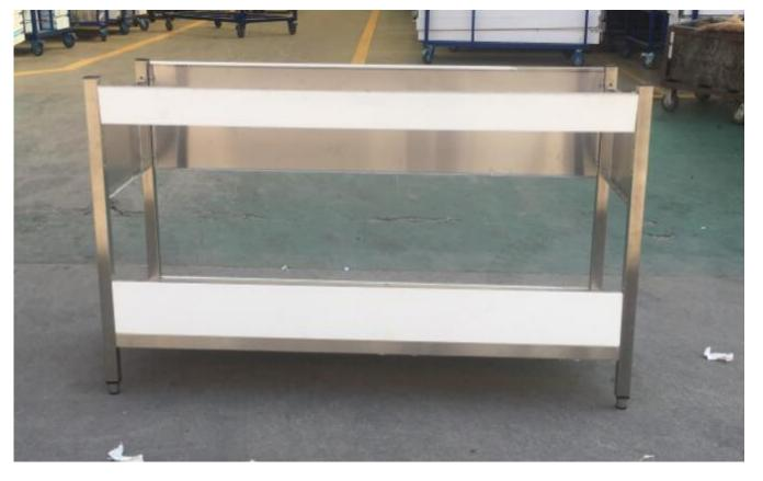
Stop 02:Install all the panel .(one left panel,one right panel,one front panel and two back panel )Please use a small wrench to tighten 10 screws of M6.
