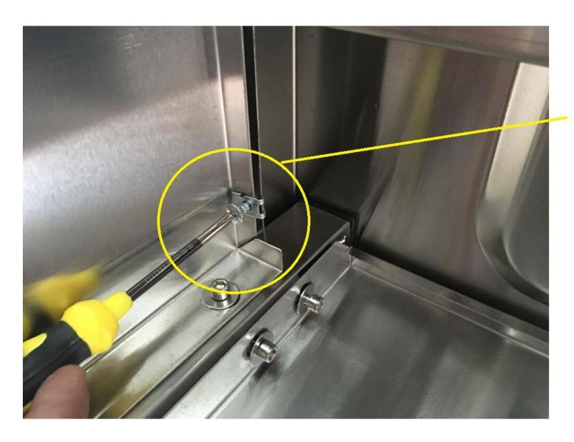
Use the screw driver to fix the screw and the gasket for sink top and left panel, make it very tight.
